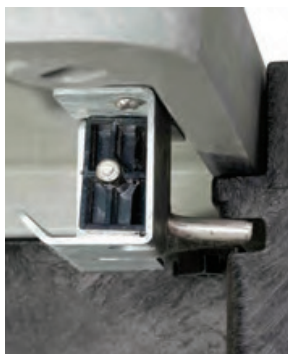
L-Bolt Security System (SHIELD Cover Shown)
